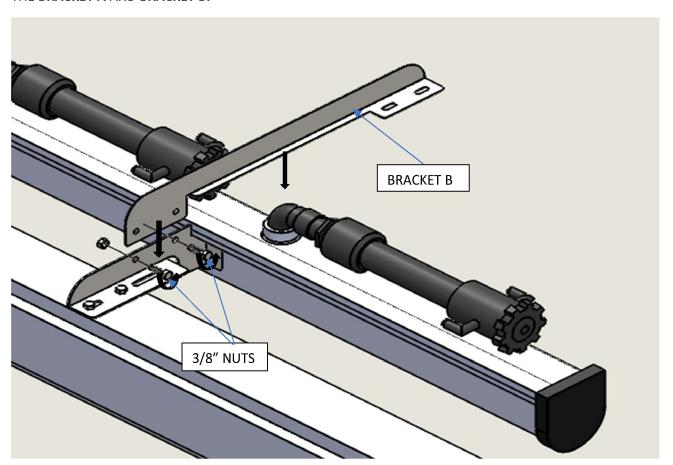
STEP 5: ALIGN THE HOLES ACROSS OF THE LED HINGES AND BRACKET B TIGHTEN THE NUT AND BOLTS.
