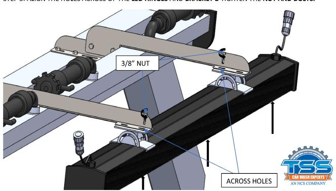
STEP 6: REPEAT THE PROCEDURE BY TIGHTENING THE REMAINING HOLES.
