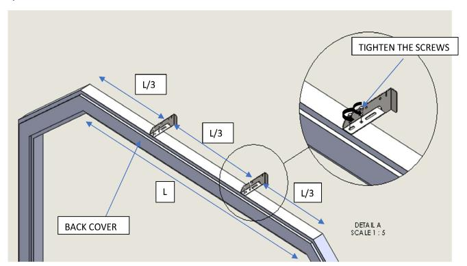
STEP 3: PLACE THE TUBE APPLICATOR ON TOP THE BRACKET A BY ALIGNING THE NOTCHES.
