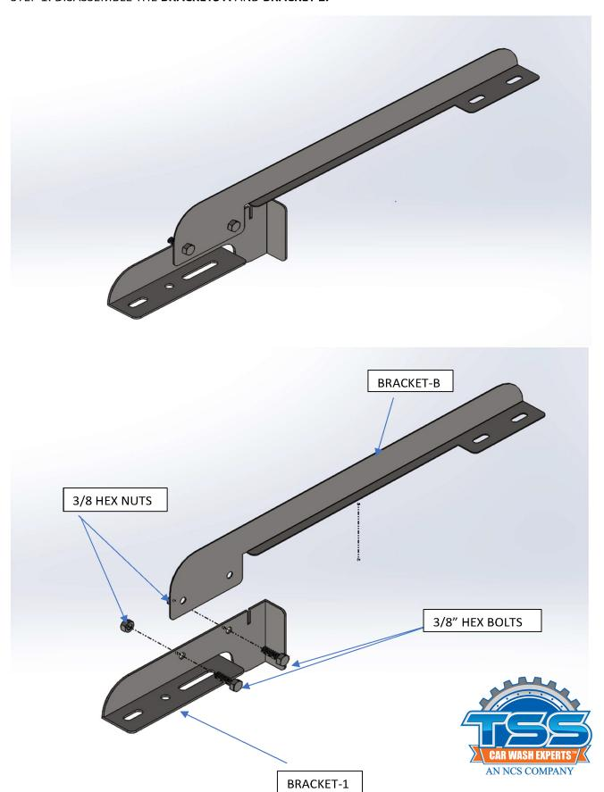
STEP 2: OPEN THE BACK COVER OF THE ARCH AND TIGHTEN THE **BRACKET A** ON TO THE ARCH WITH **3/8" BOLTS**.
