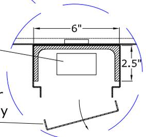
**Aluminum used:** Structural components are made of Alloy 6061-T6 / Shell is made out of 3105-H14 baked enamel.
